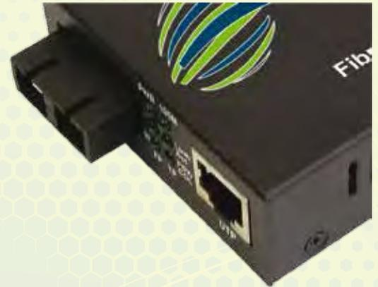
Media Converters provide an intelligent solution for fibre optic connectivity where simplicity, low cost, and minimum footprint are the primary considerations. The converters are designed to handle both legacy 10BaseT and 100BaseTX Fast Ethernet devices on their twisted pair port while maintaining 100BaseFX Fast Ethernet transmission on the fiber optic port. Plug-and-play simplicity makes connection easy.
